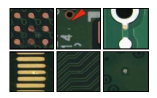
After drilling copper-clad laminates, this system inspects for defects such as missing, oversized, undersized, or multiple holes, as well as debris in round and slotted
